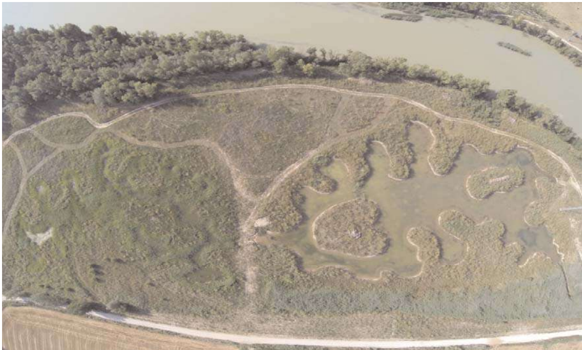
Figure 6. Creation of a new wetland adjoining the Aragon River at Soto Manolo (Caparroso). This project involved the elimination of a commercial poplar plantation and the creation of an irregular shaped basin receiving excess water from irrigation. Extremely diverse shallow and semi-flooded aquatic habitats highly suitable for the European mink have resulted.
