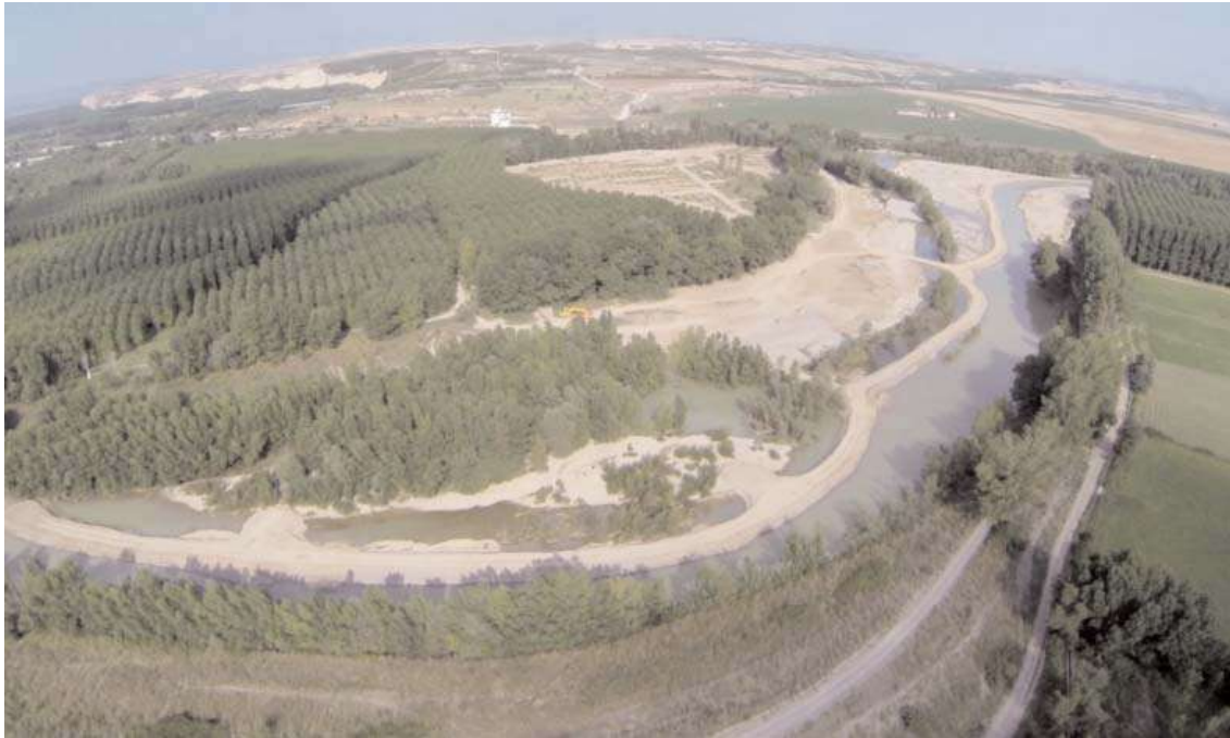
Figure 2. Two views of the Sotocontiendas project (Marcilla). The first picture shows the two kilometres of platforms made using gravel removed from the banks and arranged in order to be returned to the Aragon River when the water level rises. The second picture shows the area recovered for the river once earth embankments had been set back and the banks reshaped.
