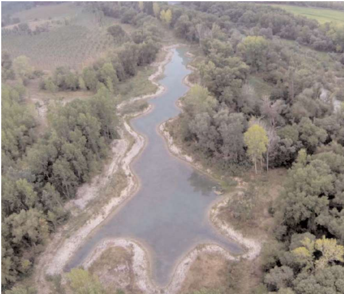
Figure 8. Wetland adjoining the Aragon created at Soto Sequero (Mérida). This wetland was created at the site of an old poplar grove and is fed by groundwater and subjected to the flow of the river system after setting back an existing defensive earth embankment.
