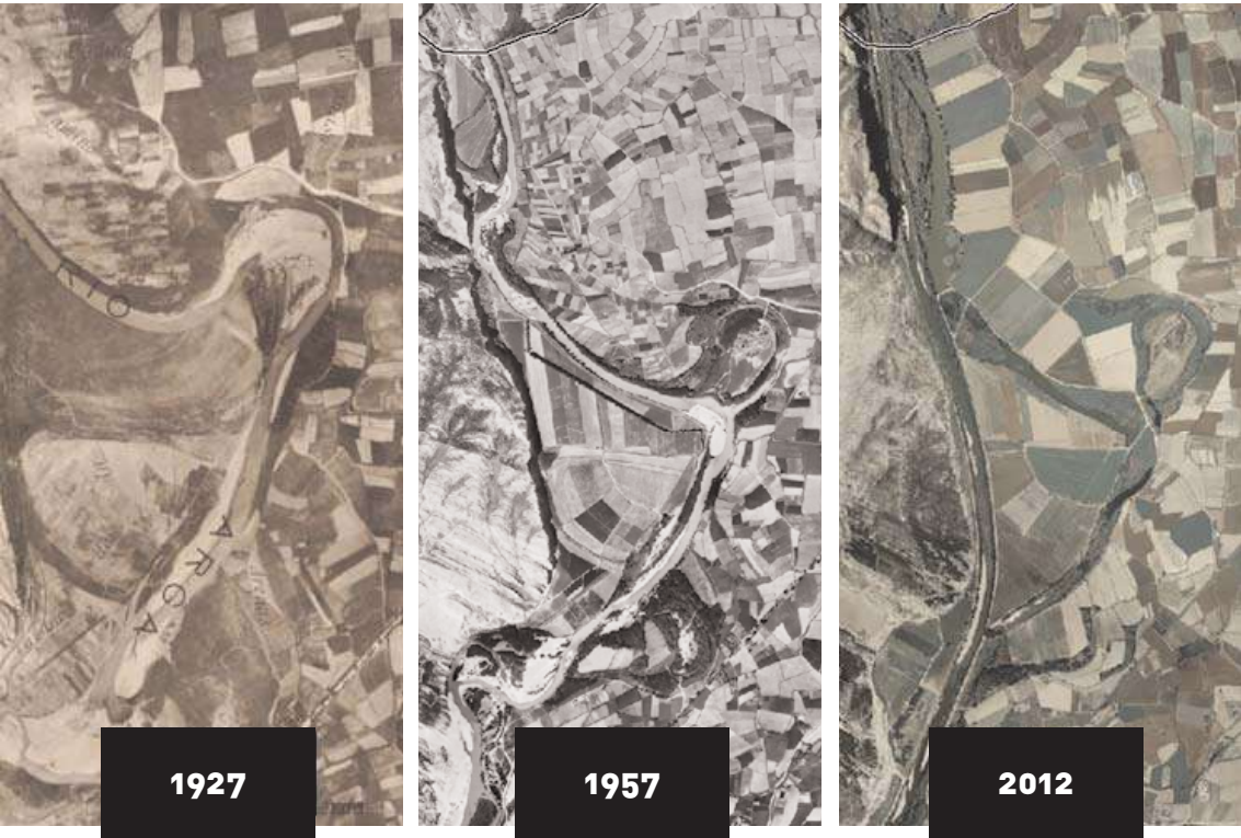
Figure 4. Development of the course of the Arga River. The picture taken in 1957 shows how the Santa Eulalia meander was naturally separated from the channel. The picture from 2012 shows the “cut-off”, which consisted of the creation in the 1980s of an artificial channel. The stretch of the Arga River shown in the pictures went from a meandering form measuring 5 kilometres in 1957 to a straight course measuring 3.6 kilometres.
